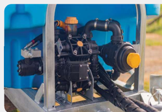
HYDRAULICALLY DRIVEN DIAPHRAGM PUMP
